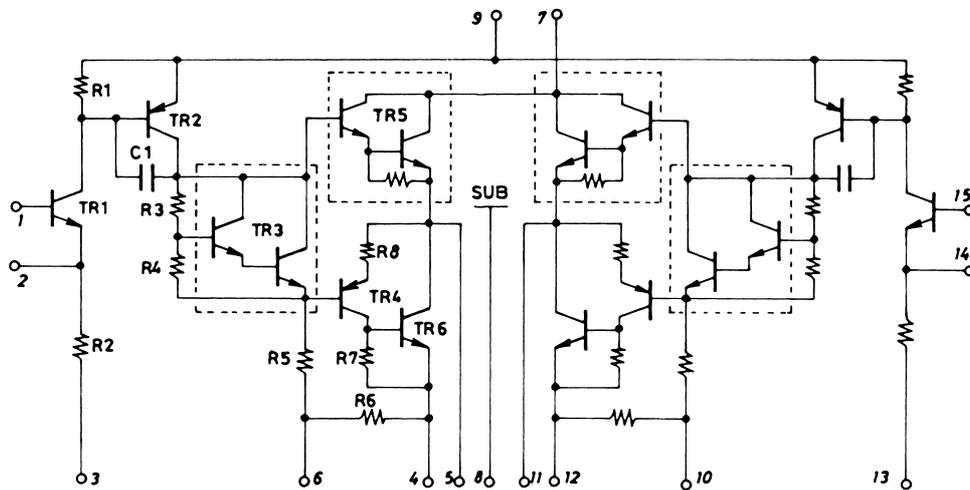
Sample Application Circuit: 10W min 2-channel AF power amplifier
